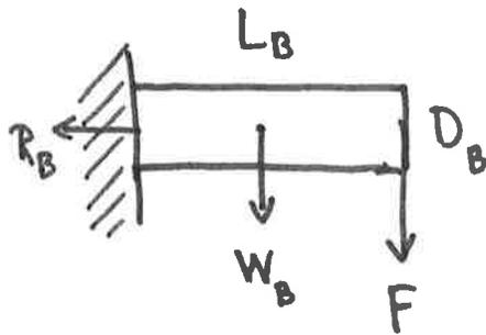
Force  $F$  applied to end of limestone pillar so that it's about to break.
