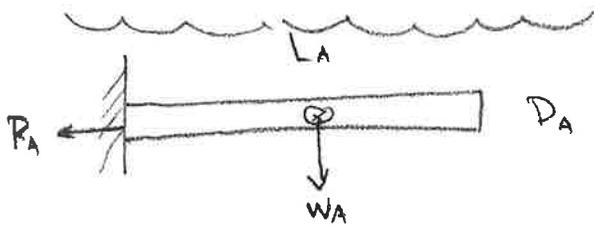
This is a submerged beam about to break under its own weight.  $L_A = 20 \text{ feet}$
