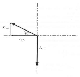
$$\begin{split} F_{ab,\,x} &= 0 \text{ N} \\ F_{ab,\,y} &= -1.73 \times 10^{12} \text{ N} \\ F_{ac,\,x} &= F_{ac} \times (-1) \cos 30^{\circ} \\ &= (5.39 \times 10^{11} \text{ N}) \times (-0.866) = -4.67 \times 10^{11} \text{ N} \\ F_{ac,\,y} &= F_{ac} \times \sin 30^{\circ} = (5.39 \times 10^{11} \text{ N}) \times (0.5) \\ &= 2.70 \times 10^{11} \text{ N} \end{split}$$
