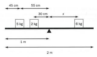
Always draw a sketch of the system in these problems. Because mass 1 and mass 2 are both on the left side of the fulcrum, mass 3 must be on the right side to balance them out. Label the distance from the fulcrum to mass 3 as x.
