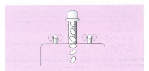
Water is dripping from a leaky faucet. As the drops fall, they oscillate as shown in the diagram above. Given that the frequency depends only on the surface tension T of the water (measured in N/m), the radius of the drops r, and the density of the water, use dimensional analysis to find a proportionality expression for the frequency f of the drops.
